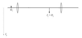
A telescope can also be constructed of an objective that produces a real image, which is then observed with a magnifying glass. There
