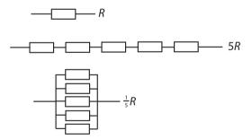
In general then we can write  $R = \rho \frac{L}{A}$ , showing the length and area dependences. The remaining factor,  $\rho$  (Greek *rho*), depends only on the material of the wire and its temperature. It is called the *resistivity*.
