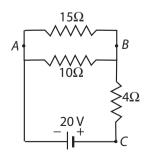
(a) What is the equivalent resistance of the 15  $\Omega$  and the 10  $\Omega$  resistors between points *A* and *B*?
