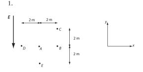
There is a uniform electric field of 3 N/C in the (-y) direction, as in the figure. Take the point *A* as a reference, with *V* = 0. What is the potential at points *B*, *C*, and *E*?
