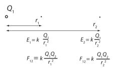
The magnitude of the field created by  $Q_1$ is  $k\frac{Q_1}{r^2}$ , and the magnitude of the force on  $Q_2$ is  $k\frac{Q_1Q_2}{r^2}$ . We want to calculate the work done as we move the charge  $Q_2$  closer to  $Q_1$ , from a distance  $r_2$  to a smaller distance,  $r_1$ .
