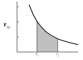
A little calculus, and the use of the expression for the integral of  $r^n$  that we cited near the end of Chapter 3, allows us to get away from guesses and approximations. For a constant force the work is equal to the force times the displacement. This is equal to the area under a curve of force against displacement. It is still the area
