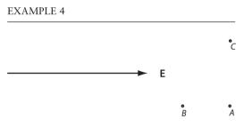
There is a uniform field of 5 N/C in a region. A charge of  $2 \times 10^{-4}$  C is moved from a point *A* to a point *B* along an electric field line in the direction opposite to the field, a distance of 3 m.
